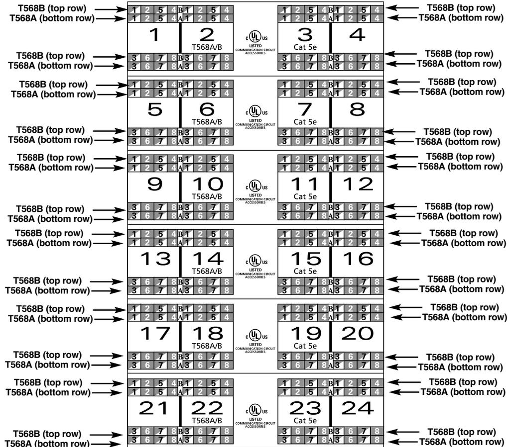
Figure 5. 24-port patch panel's T568B and T568A wiring labels.
