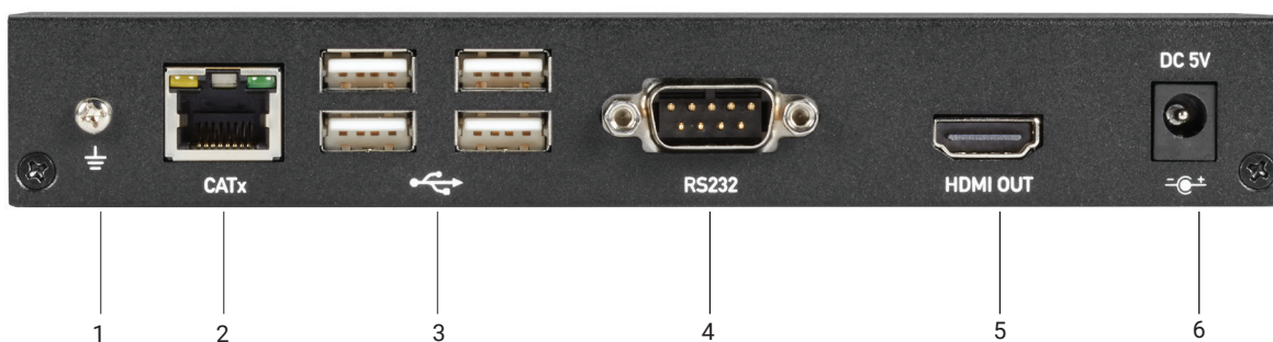
FIGURE 2-13. SINGLE-HEAD CATX RECEIVER BACK PANEL
